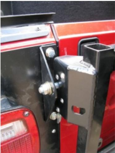
With the latch bracket in place, adjust the position of the pin so that it completely engages the latch mechanism. Additionally, the tire carrier should sit loaded against the rubber stopper on the bumper. This is critical to minimize vibrations.
