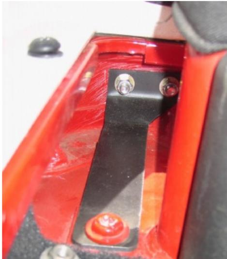
Remove the outside roll cage bolt. Install the upper hinge backing plate as shown using two of the 3/8" bolts and supplied flat washer and lock nuts.
