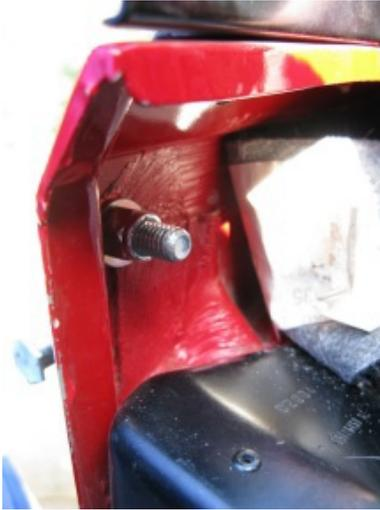
Insert three of the 3/8" x 1.25" bolts with flat washers. Tighten the upper bolt with a flat washer and lock nut.
