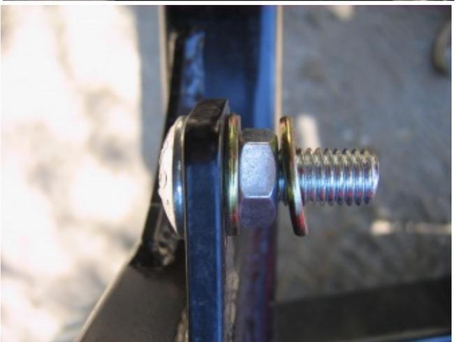
Locate and install the 1/2" carriage bolt through the 2 lower Hi-Lift tabs. Install a flat washer and included jam nut (thin hex nut). The Hi-Lift will mount to this stud and secure with a wing nut on the outside.
