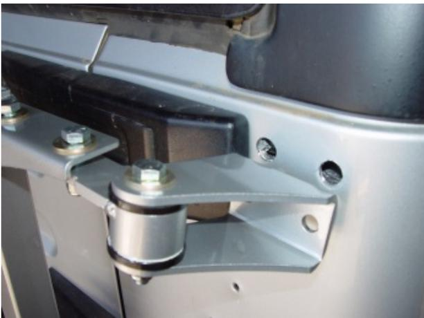
Bolt the upper hinge arm to the tire carrier using two of the 3/8" x 1.25" bolts and corresponding flat washers and lock nuts.
