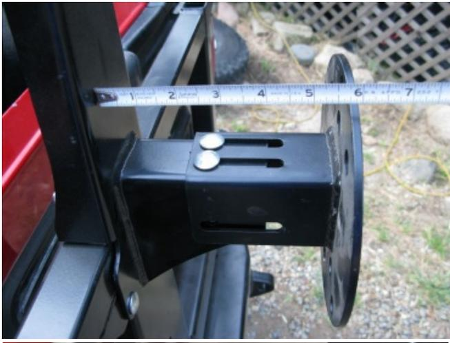
Using the measurement from the previous step, measure and adjust the wheel hub and antenna post to the right offset. The wheel hubs will secure to the antenna post using the 5/16 x 3/4 carriage bolt, flat washers and lock nuts.
