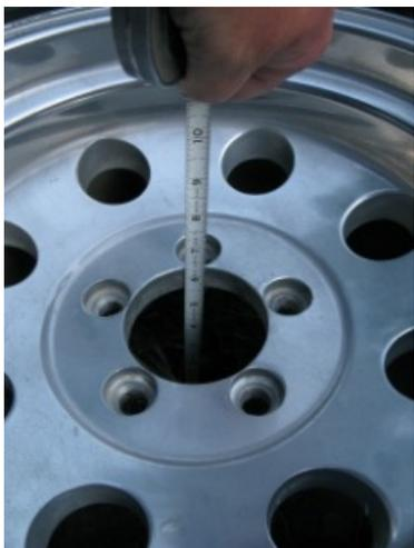
Using the spare tire, set the rim down on a flat surface and measure to the backside of the rim. Subtract 3/4" and use this measurement in the next step.
