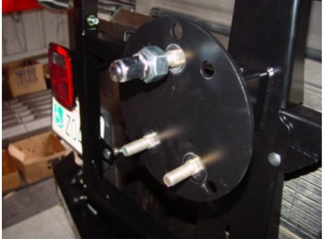
NOTE: This step can be complete with a basic h-frame press, securely mounted vice or while installed on the tire carrier.
