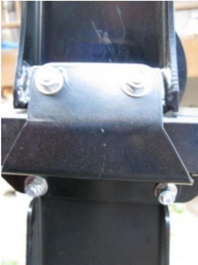
Mount the antenna post to the center of the tire carrier using the antenna post backing plate as shown to brace the entire assembly. The top two holes will use the 5/16" x 3/4" bolts and the bottom will use the 5/16" x 1" bolts..
