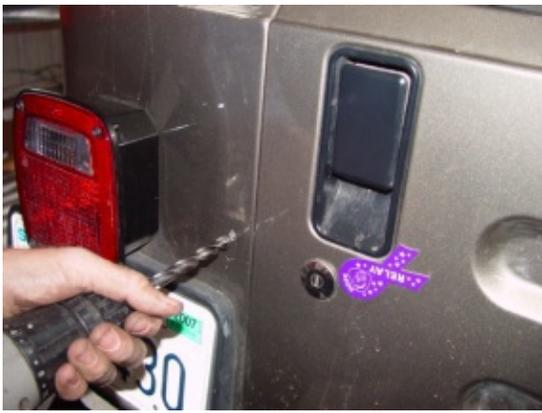
Drill through the tub with a 1/4" pilot bit. Once all three holes have been started, open them all up using a 7/16" drill bit.
