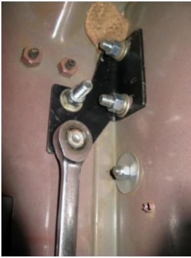
Insert two of the 3/8" x 1.25" bolts with the flat washers from the cargo area into the rear fender well. Tighten the two bolts in the fenderwell with supplied flat washer and lock nuts.
