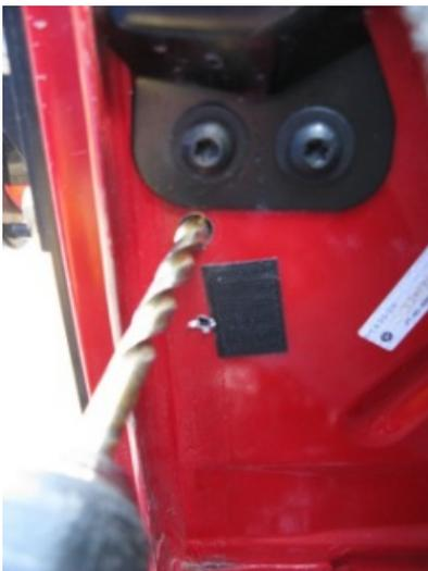
Drill through the piloted holes with a 7/16" drill bit as shown in the photo
