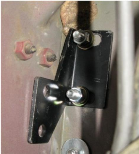
Install the latch bracket backing plate inside the fenderwell as shown using two of the supplied 3/8" bolts, washers, and lock nuts. Then pull back the carpet from the cargo area and pilot the holes in the bracket through to the cargo area.
