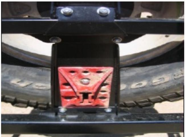
Before installing the Hi-Lift jack to the tire carrier, remove the foot pad and secure to the antenna post using a 5/16" x 1" carriage bolt through the center as shown in the photo.
