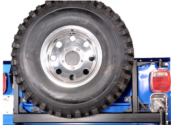
Portions of the tire carrier, and corresponding rear bumper come with parts pre-installed by Hanson Offroad. The rear spindle bumper (JRR4102-P) will have the latch pin, scuff block, spacer plates and rubber stopper installed. The tire carrier (CTC2-P) will have the spring loaded locking pin assembled on the pivot side of the carrier and the upper latch installed on the opposite side. The upper tub bracket will have the latch pin installed as well.
