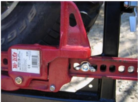
Mount Hi-Lift Jack to the lower tabs on the tire carrier using the included 1/2" carriage bolts, flat washers and wing nut.
